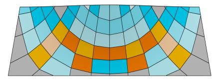
**Figure 8:** Illustration of the mold depot and the cost model by means of the example shown in Figure 3(e). The colors of panels are saturated according to mold reuse. Figure 4 lists the glass cost ratios used for this example.
