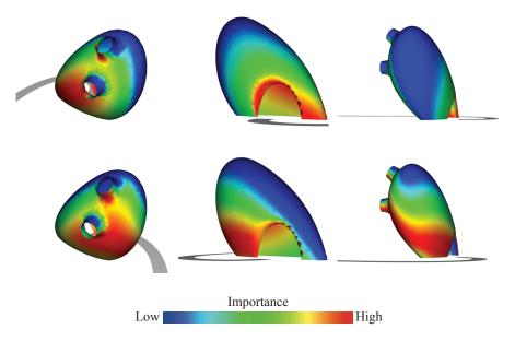
(a) Spatially adaptive importance functions computed based on visibility from path 1 (top row) and path 2 (bottom row). These importance functions are used for paneling solutions as shown in 10(b) and Figures 11-13 (b) and (c), respectively.
