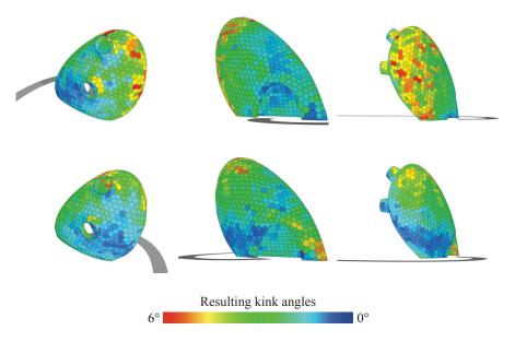
(b) Kink angles of two paneling solutions (top and bottom rows) using adaptive thresholds based on the two importance functions shown in 10(a). Further renderings of the results are shown in Figures 11-13.
