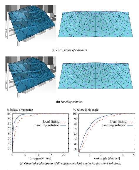
**Figure 9:** The paneling algorithm restricted to cylindrical panels. Here we compare a result on the Facade Design Study computed using simple local fitting of cylinders (a) to a paneling solution using only cylinders (b). For both results we show the axis directions of cylinders colored in magenta and the cumulative histograms of resulting divergences and kink angles.
