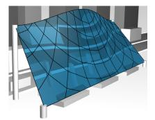
(c) Paneling solution using 1° kink angle threshold (divergence: 4.7mm; cost: 294).
