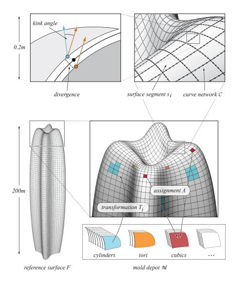
**Figure 5:** Terminology and variables used in the paneling algorithm. The reference surface F and the initial curve network C are given as part of the design specification. The optimization solves for the mold depot  $\mathcal{M}$ , the panel-mold assignment function A, the shape parameters of the molds, the alignment transformations  $T_i$ , and the curve network's normal displacement. Figure taken from [Eigensatz et al. 2010].
